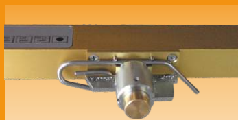
Adapter for checking switch blades (optional)
